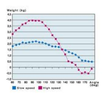
Weight stack machines are more suited to slow, controlled movements. An increase in speed produces inertia, distorting the loading on the muscle, impacting on the joint and reducing the training effect.
